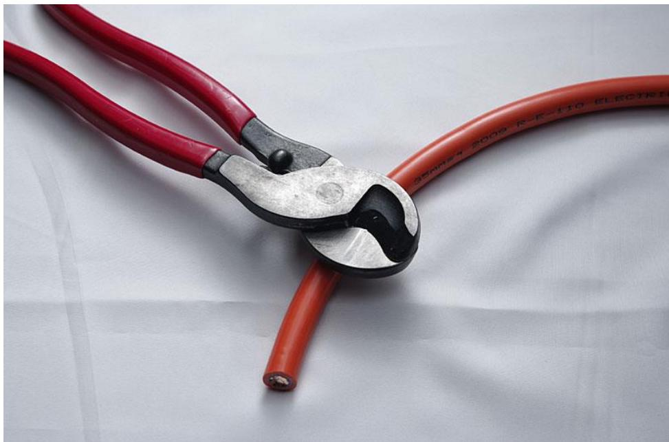
**Step 2** – Strip the insulation to the correct distance for the crimp you are using. When inserted into the crimp, the insulation should touch the barrel of the crimp with no large gaps and you should be able to see the ends of the copper strands through the inspection hole next to the lug of the crimp.
