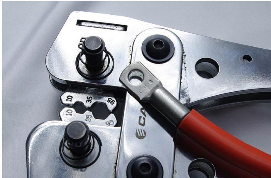
**Step 5** – Set your hex crimp tool to the same size as the crimp lug. In the example photos here, we have used 35mm<sup>2</sup> cable, lugs, and crimp tool. To crimp with the proper force, you will need either a 'bolt cutter' type crimp tool, as shown in the photo above, with handles around 600mm (2') long, or a hydraulic tool with an appropriate crimp die set.
