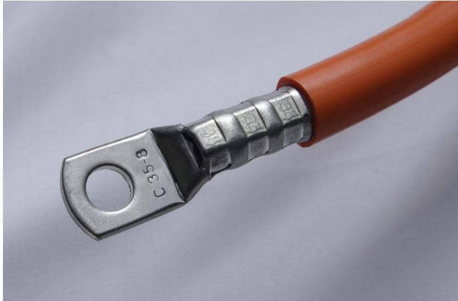
**Step 6** – Crimp the barrel of the crimp. For the tool used in these photos, it can be crimped three times along the length of the barrel. A hydraulic tool may be similar. A high volume tool will probably only require a single action.
