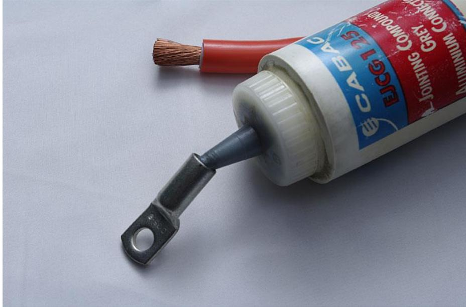
**Step 4** – Insert the wire into the crimp. Hold your finger over the inspection hole to stop the jointing compound coming out, therefore forcing it up between the wire strands. Push the wire all the way into the crimp barrel, so that the wire insulation touches the end of the barrel with no large gaps.
